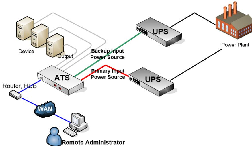
**Best configuration:** Redundant Switch with two Smart-UPS units connected to two separate AC lines, each UPS receiving power from a separate facility power source.
